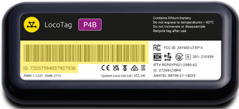
Fig 2. An image of the LocoTag P4B with the device ID and barcode highlighted.
