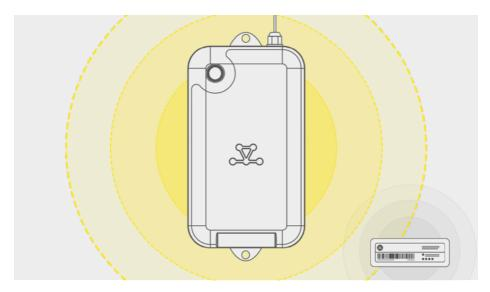
Any activated LocoTag or LocoTrack configured as a Tag will begin reporting through the switched on LocoTrack HFR4 as soon as they come into range, 20m (65.6ft) indoors and 80m (262.5ft) outdoors.
